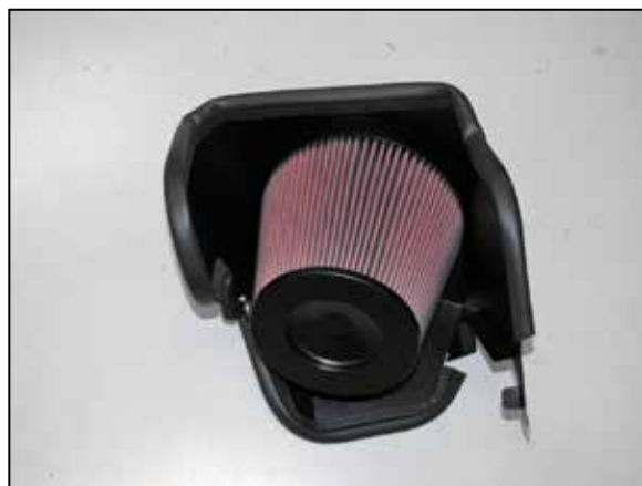
13. Install the K&N® air filter onto the filter adapter and secure with the provided hose clamp. NOTE: Drycharger® air filter wrap; part # RC-5139DK is available to purchase separately. To learn more about Drycharger® filter wraps or look up color availability please visit http://www.knfilters.com ®.
