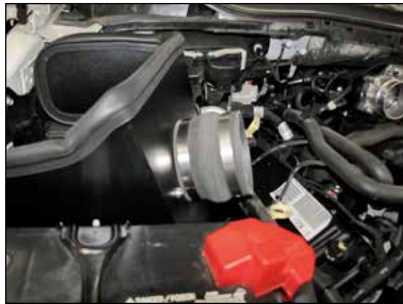
15. Install the provided hump coupler (08418) onto the filter adapter and secure with the provided hose clamp.
