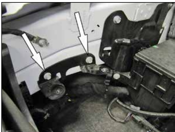
7. Remove the two bolts that secure the air filter mounting bracket to the fender and then remove the bracket from the vehicle.
